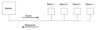
In the MODBUS Protocol the master can address individual slaves, or, using a special "Broadcast" address, can initiate a broadcast message to all slaves. The Triload Digital meter does not support the broadcast address.
